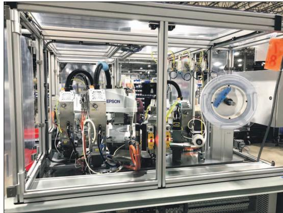
AGR designed, built and installed this machine that makes part of COVID test kits.
